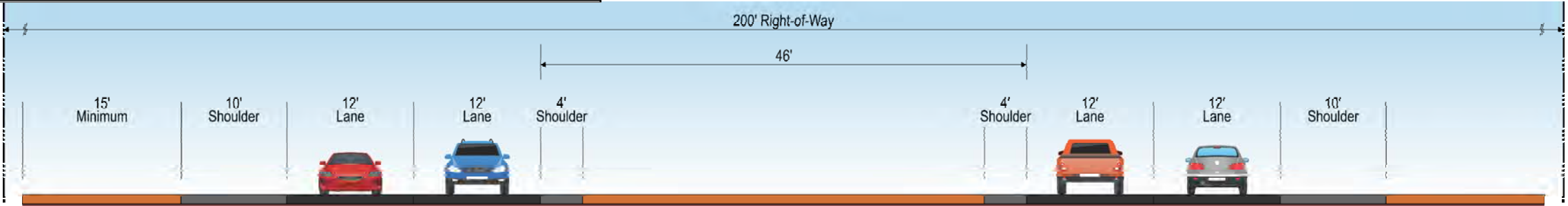
Fringe-Urban Highway Typical Section Figure 306.3 in ADOT RDG
